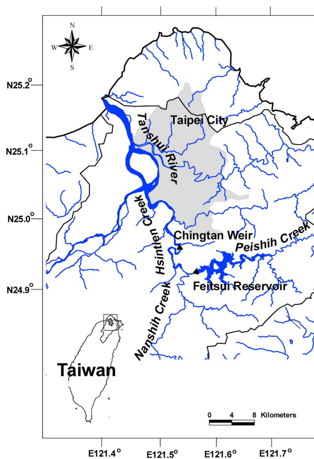
Figure 1. Location map of Feitsui Reservoir system and Hsintien Creek basin. The joint flow from the Peishih and Nanshih Creeks is diverted at the Chingtan Weir to supply the domestic demand of the Taipei metropolitan area.
