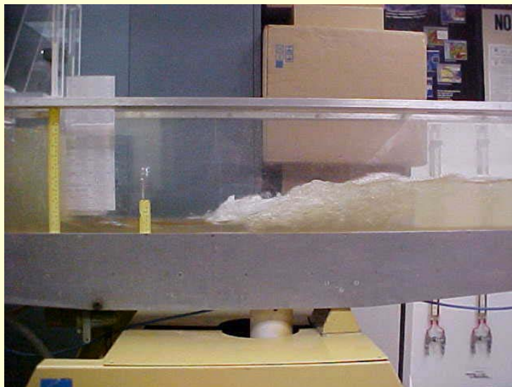
Hydraulic jump in a laboratory flume (實驗水槽)
